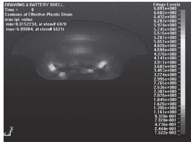
Fig. 5 Effective strain in Ni coating with a punch stroke of 10 mm
